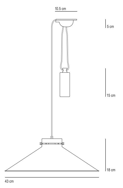
Cable length may be shortened upon installation. This will reduce both maximum & minimum drop and reduce the range of movement.
